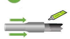
Similar to cold shrink, these products are made of elastomeric material. Since these are supplied in unexpanded form the shelf life is unlimited.
