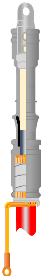
Moulded body without creepage sheds for indoor dry box
